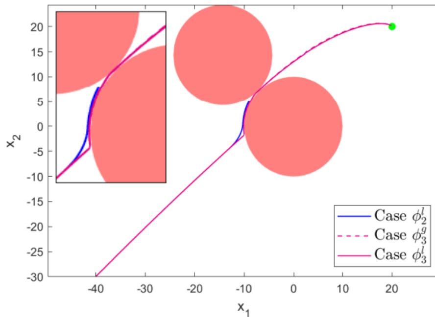
Figure: A simulation with two tightly-spaced obstacles, in which controllers using margins  $\phi_3^l$  and  $\phi_3^g$  permit passage through the obstacles, while the other functions force the agent to stop.
