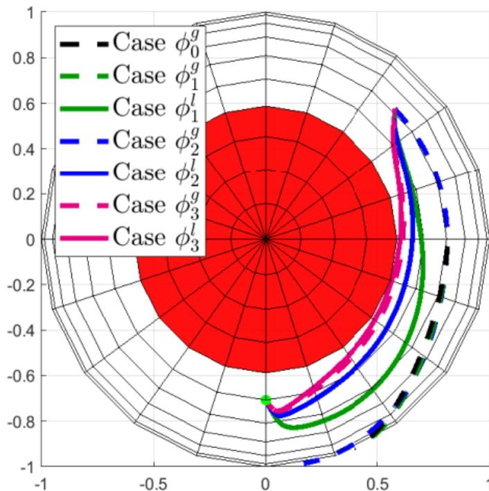
Figure: Trajectories of the spacecraft attitude system for all 7 margin functions
